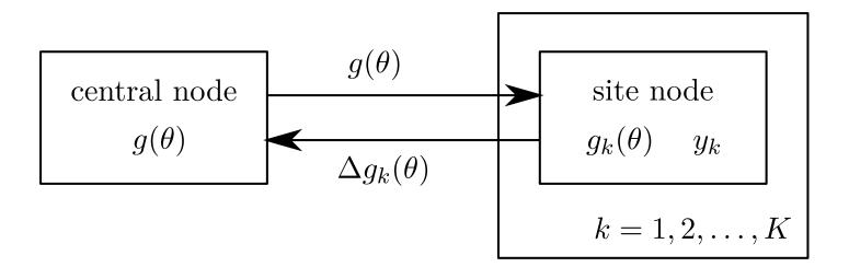
Figure 1: The EP framework for partitioned data. The central node stores the current parameters for the global approximation  $g(\theta)$ . Each site node  $k = 1, 2, \ldots, K$  stores the current parameters for the site approximation  $g_k(\theta)$  and the assigned partition of the data  $y_k$ . The central node sends the parameters of  $g(\theta)$  to the site nodes. In parallel, the site nodes update  $g_k(\theta)$  and send back the difference in the parameters.
